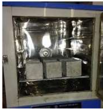
Figure 6: Oven curing of specimens at 60°C for 24 hrs
