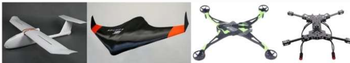
Different airframes. From the left: polystyrene, plastic, aluminum, carbon fiber
