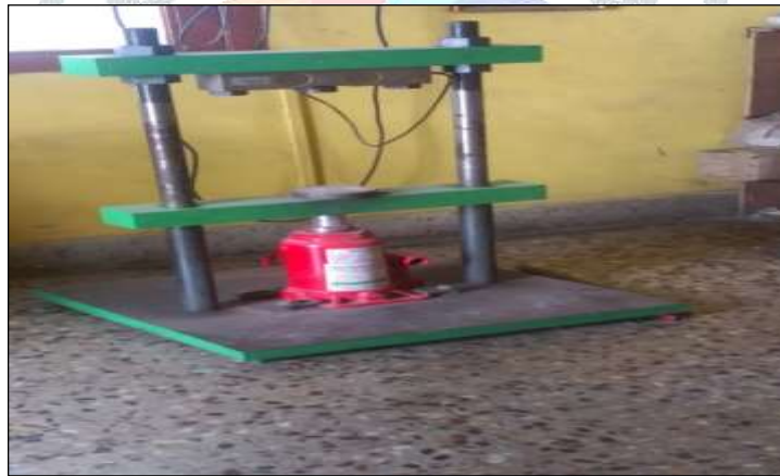
Figure-2: Compaction Machine
