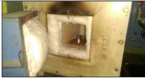
Figure-4: Sintering Furnace
