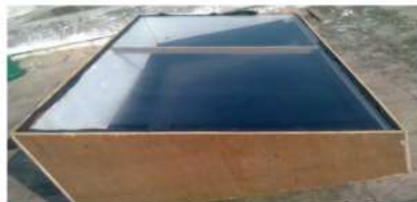
Fig 1: Single basin single slope setup
