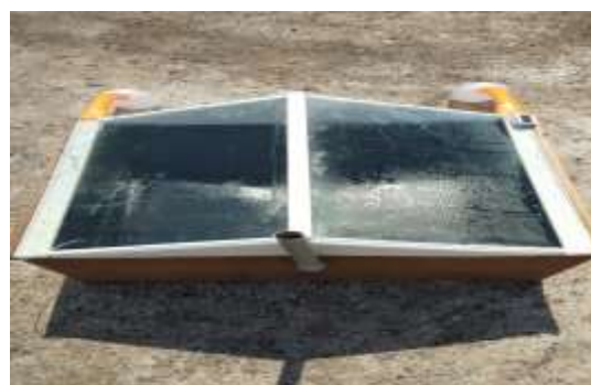
Fig 2: Single basin Double slope setup
