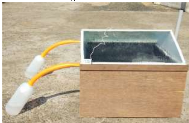
Fig 6: Solar still with PCM setup
