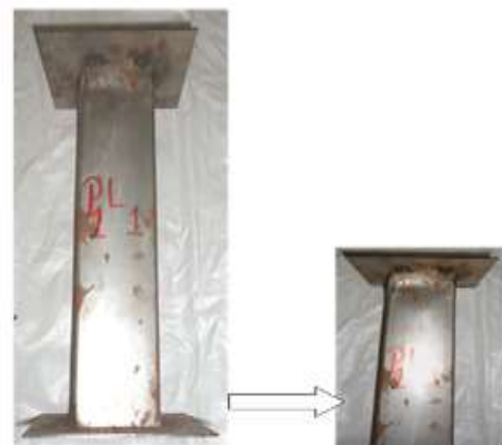
Fig. VIII. Specimen P_1L_1 buckling mode
