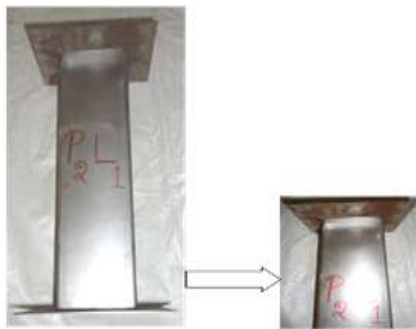
Fig. X. Specimen P_2L_1 buckling mode
