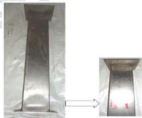
Fig. XIV. Specimen P_2L_1B buckling mode
