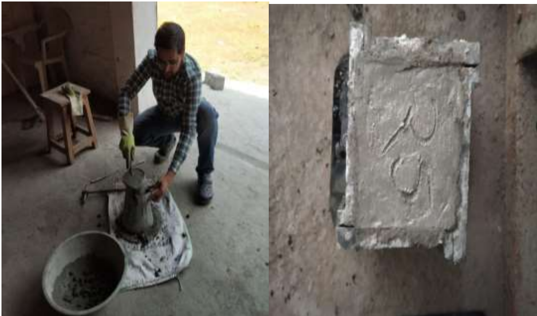
Fig 3: workability by compaction
