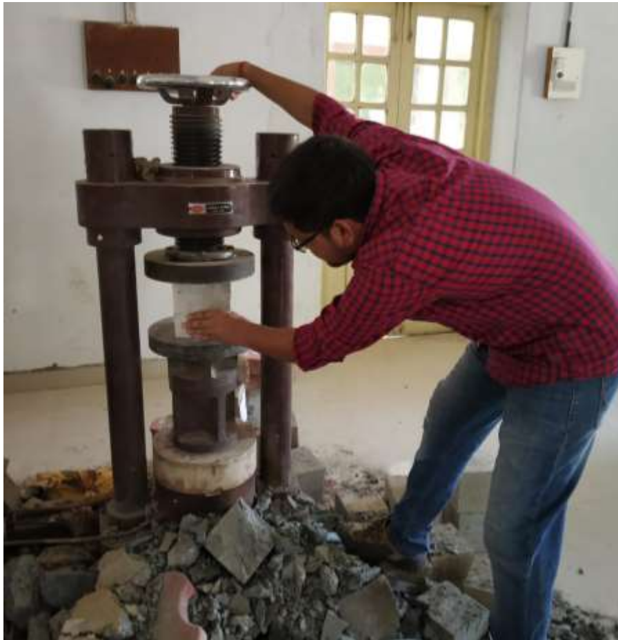
Fig 4: Compression Testing of Cube Specimen
