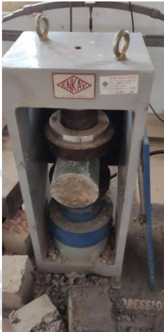
Fig:5-Split Tensile Testing and Specimen Experimental Results
