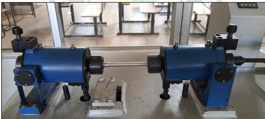
Figure 2: RR Moore fatigue testing machine
