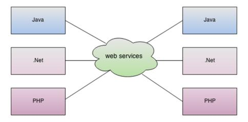
In the above diagram Java, .net, and PHP applications can communicate with other applications through web service over the network.
