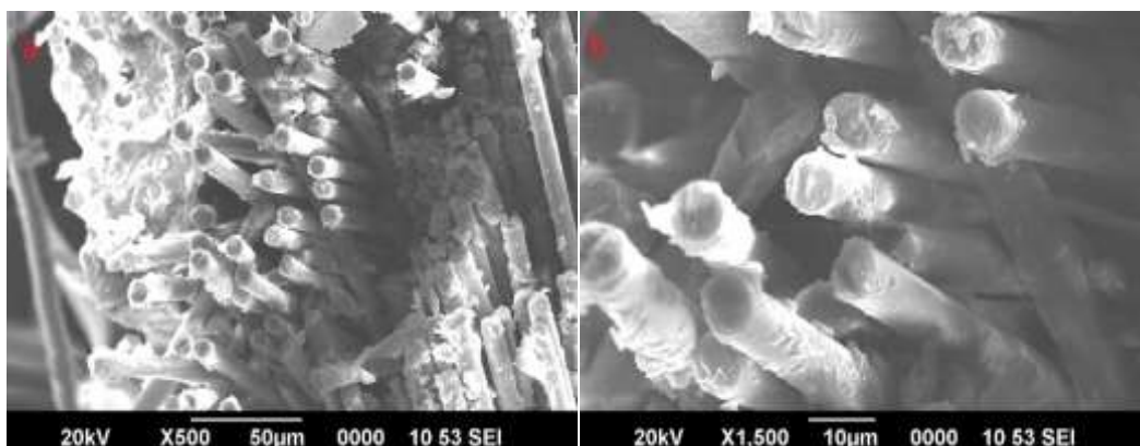
Figure 21 Fracture surface of 1% Cloisite15A filled sample under tensile load of CHS 50 mm/min
