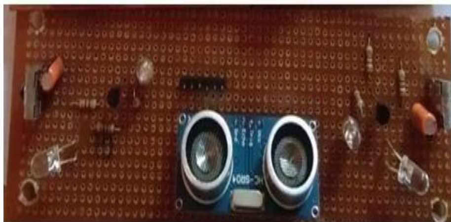
Fig. 5 Connection Ultrasonic Sensor & Infrared Sensor
