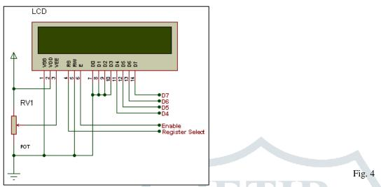
Here only D4, D5, D6 and D7 data pins are used and D0, D1, D2 and D3 are kept grounded.
