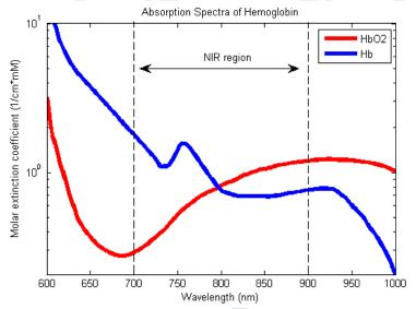
The oxygen content can then be calculated easily by comparing the how much red light is absorbed as compared to infra-red light.
