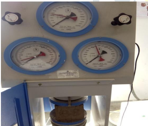
Fig.1: Test Setup to check compressive strength of cube
