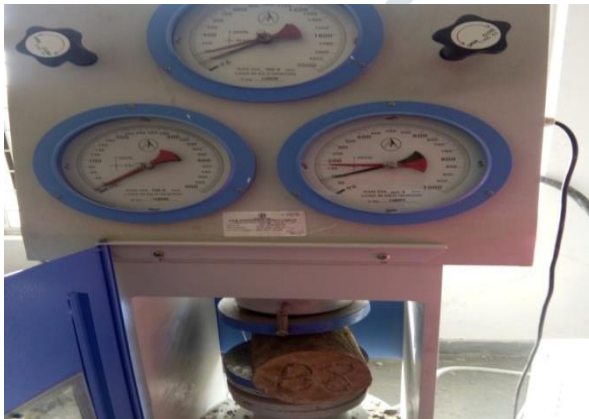
Fig.3: Test Setup to check split tensile strength of cylinder
