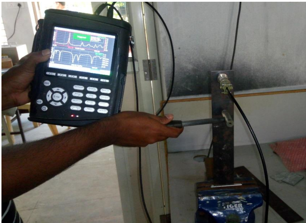
Fig.4.1 Modal test setup
