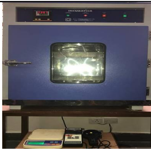
Figure 1: Drying Incubator, weighing machine and anemometer.
