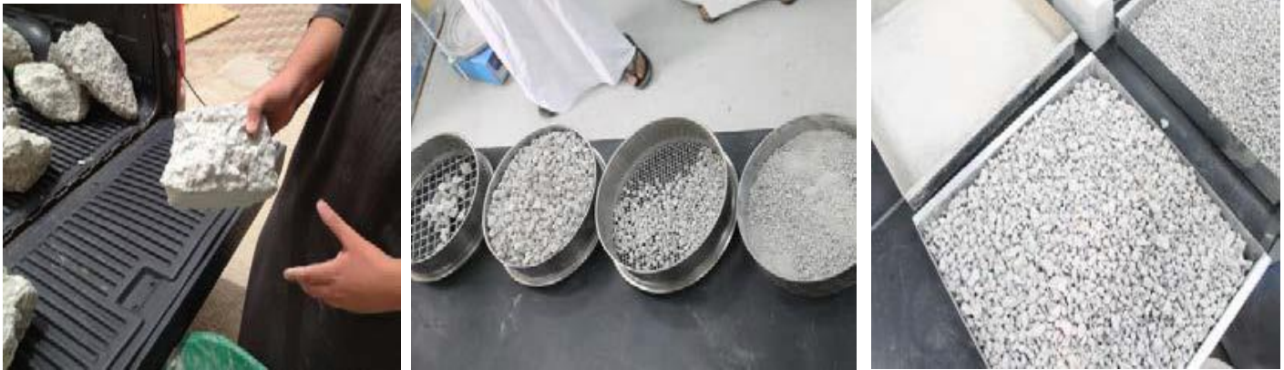
Fig 2: Processing construction debris into gravel.
