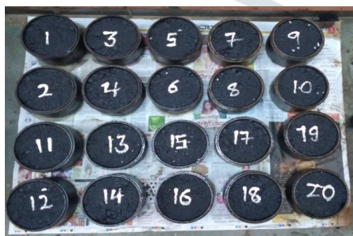
Fig. 5. Marshall test specimens
