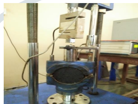
Fig. 6. Marshall test setup
