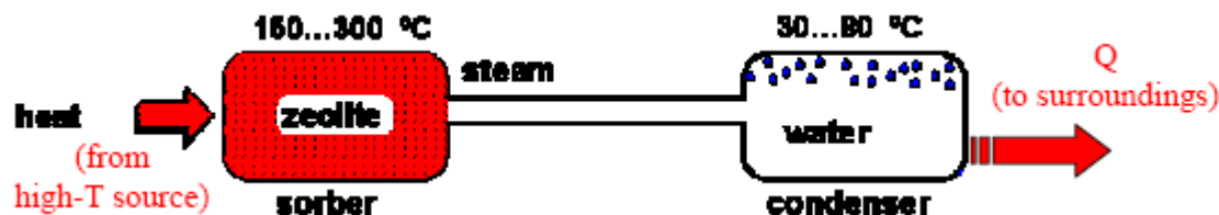
Fig: 1.2 Desorption phase of a Zeolite system
