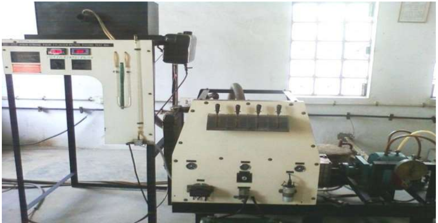
Fig. 1 Experimental Set Up for the Effect of Gasoline and Gasoline-Methanol Blends
