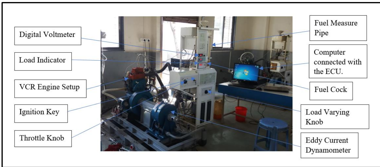
Figure 2: VCR Engine Setup with Description
