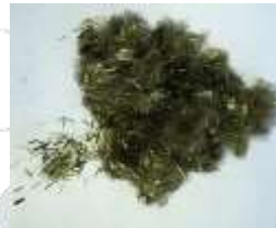
Fig. 1 Chopped Basalt Fiber
