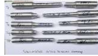
Fig.10 After Tensile Testing
