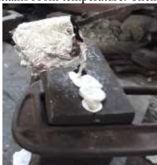
Fig. 2 Pouring Hot Mixture in Mould
