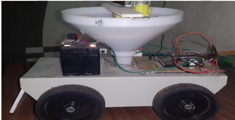
Fig.6. Actual image of prototype Automatic Seed Sowing Robot
