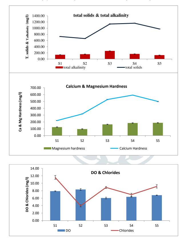
The TS of S1, S2 is within normal range i.e. 730±7.64, 664±7.21 whereas the concentration of TS in S3, S4, and
