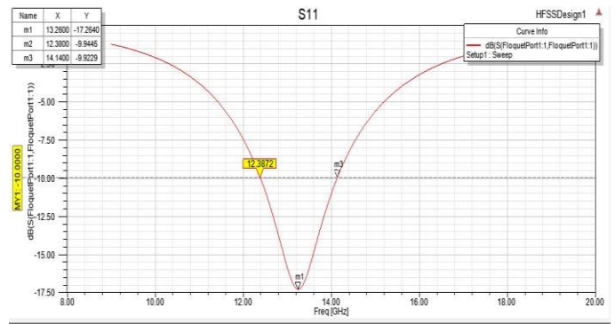
Fig 1.9 S11 or Return Loss For Proposed Antenna
