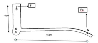
Force (Fa) required for holding the work piece is 30 N Fa = 30 N
