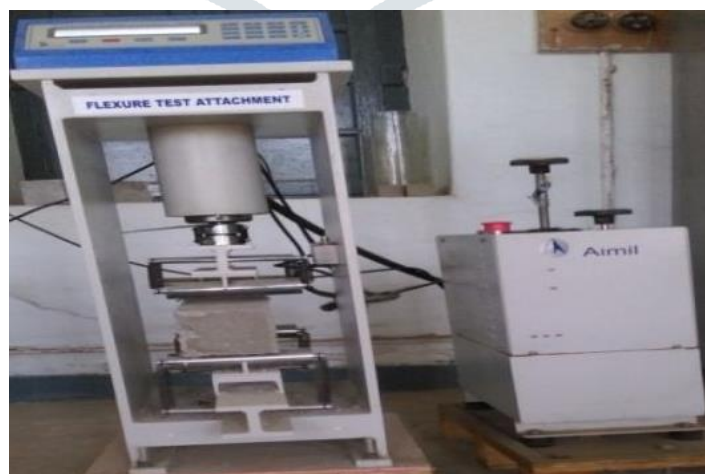
Figure 3 Flexural strength Testing machine
