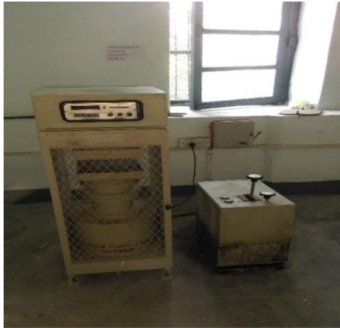
Figure 2 Setup of Compressive Strength Testing Machine
