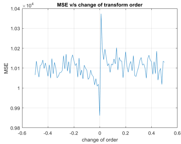
Figure 4 Variation of MSE of phase image with change in order of LCT ( \beta_3 ) remaining all Parameters constant
