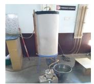
Fig 5.1: Constant Head Permeability Apparatus
