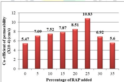
Fig 6.1: Graphical Representation of Co-efficient of Permeability with Varying Percentages of RAP
