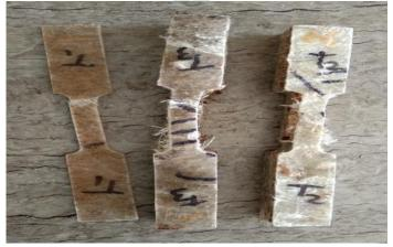
Fig10-After Tensile Test Specimen
