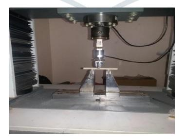
**Fig.8- Flexural Testing Machine**
