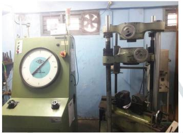
Fig.7- Universal Testing Machine
