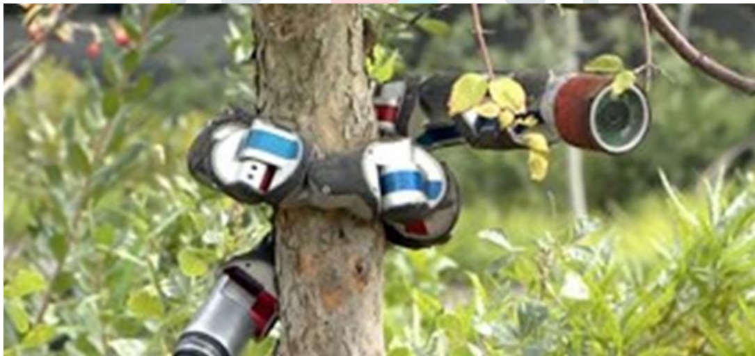
Figure. 5. The snake robot Uncle Sam developed at Carnegie Mellon University. The robot has a strong and compact joint mechanism and can climb trees. Courtesy of Carnegie Mellon University.
