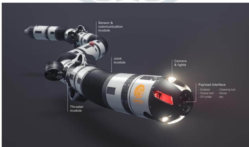
Figure. 8. Snake-like robots are gearing up to monitor the Åsgard oil and gas field off the Norwegian coast (Norwegian University of Science and Technology)
