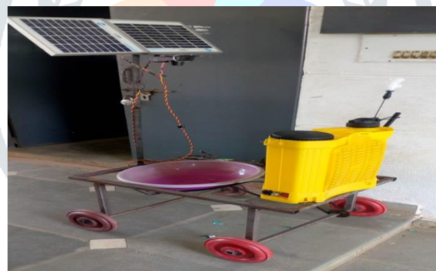
Fig 4 Frame, wheels and support structure which holds the solar panel
