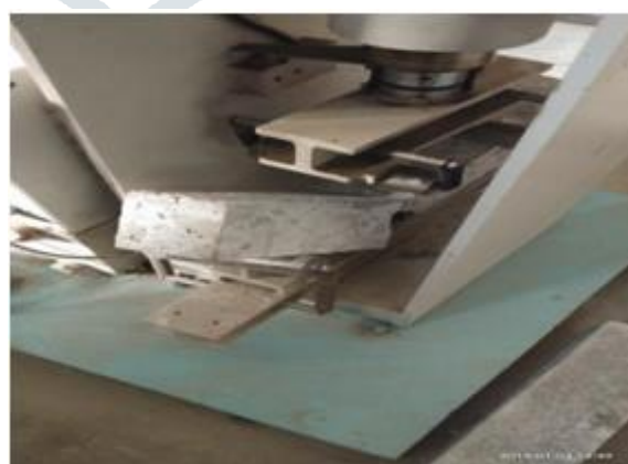
Figure 3: Failure of prism
