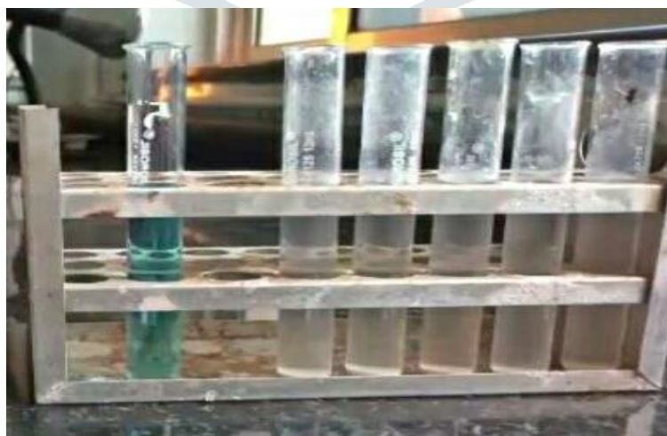
fig. 19 showing degradation of methylene blue
