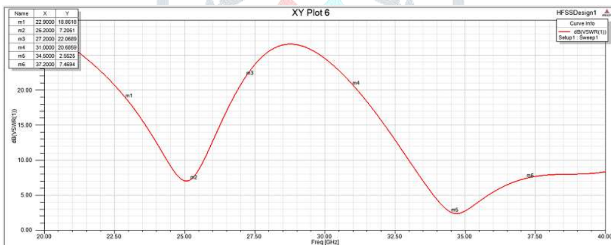
Figure 2: VSWR Plot of the Proposed antenna in Ansoft HFSS platform
