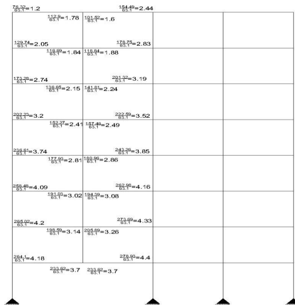
Fig. 6 Case3)Adjacent to Corner column removal
