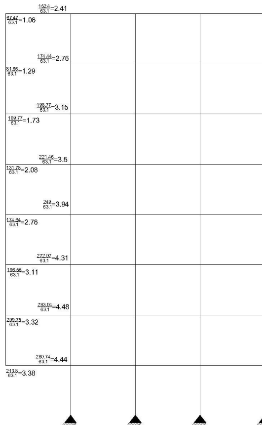
Fig. 5 Case2)Corner column removal
