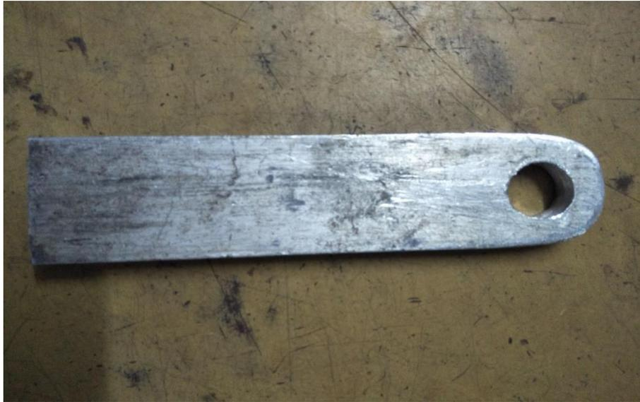
Figure 14: Fabricated lug joint
