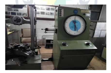
Figure 16: Universal Testing Machine
