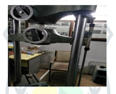
Figure 17 Lug clamped in between upper and middle cross head jaws
