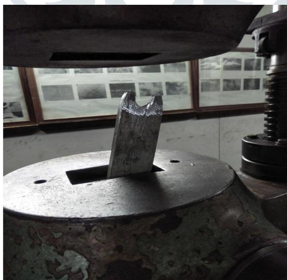
Figure 18: Fractured lug after tensile test
