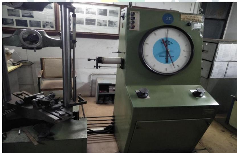
Figure 16: Universal Testing Machine
