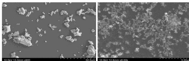
Fig- 5: SEM images of synthesized silver nanoparticles.
