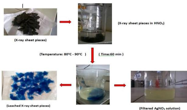
Fig -1: Flow chart for the production of silver nitrate solution
