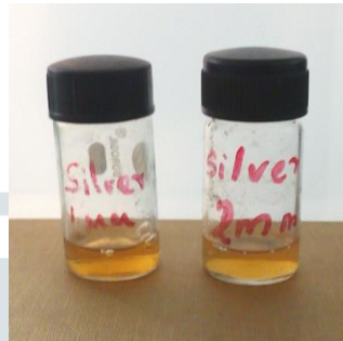
Figure 1: Appearance of dark brown color in solutions of 1mM and 2mM \text{AgNO}_3 indicating the synthesis of Silver Nanoparticles
