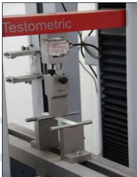
Figure 10 3-point bending test set-up
