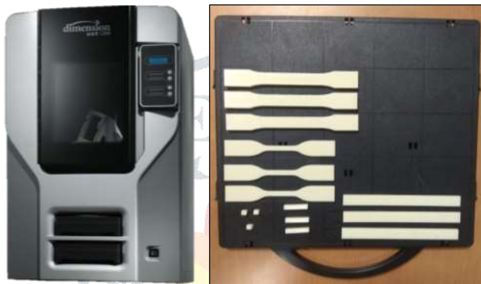
Figure 6 Dimensions SST 1200es (FDM machine) and 3D printed part
