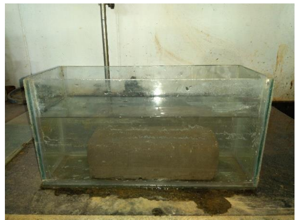
Fig.9 Water absorption test
