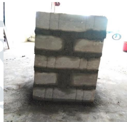
Fig.11 Hybrid ash brick masonry prism
