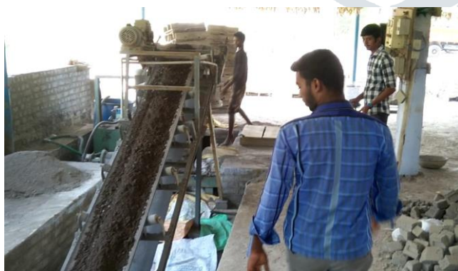
Fig.2 Transportation Of Mix Using Conveyor Belt
