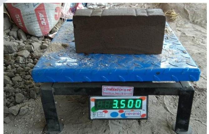
Fig.6 Wet weight of conventional fly ash brick
