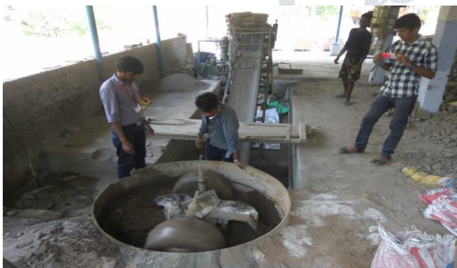
Fig.1 Brick Material Mix Using Double Drum Mixer
