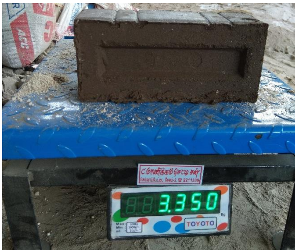
Fig.7 Wet weight of hybrid ash brick
