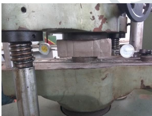
Fig.8 Compression strength test
