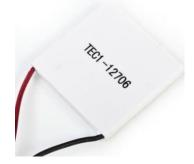
Thermoelectric cooling uses the Peltier effect to create a heat flux between the junction of two different types of materials. A Peltier cooler, heater, or thermoelectric heat pump is a solid-state active heat pump which transfers heat from one side of the device to the other, with consumption of electrical energy, depending on the direction of the current. Such an instrument is also called a Peltier device, Peltier heat pump, solid state refrigerator, or thermoelectric cooler (TEC).
