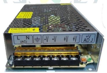
SMPS is used to provide a constant supply voltage and current to both units i.e heating unit and cooling unit. The type of SMPS we are using gives 12V 10A that means the current rating and votage rating is 12V and 10A respectively. The peltier module requires constant power supply 12V 6A which is provided through SMPS.
