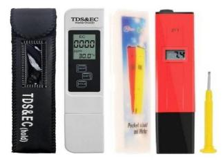
A TDS meter indicates the total dissolved solids (TDS) of a solution, i.e. the concentration of dissolved solid particles. Since dissolved ionized solids, such as salts and minerals, increase the conductivity of a solution, a **TDS meter measures** the conductivity of the solution and estimates the **TDS** from that reading.Dissolved ionized solids, such as salts and minerals, increase the electrical conductivity (EC) of a solution.The EC meter checks the electrical conductivity of the meter.
