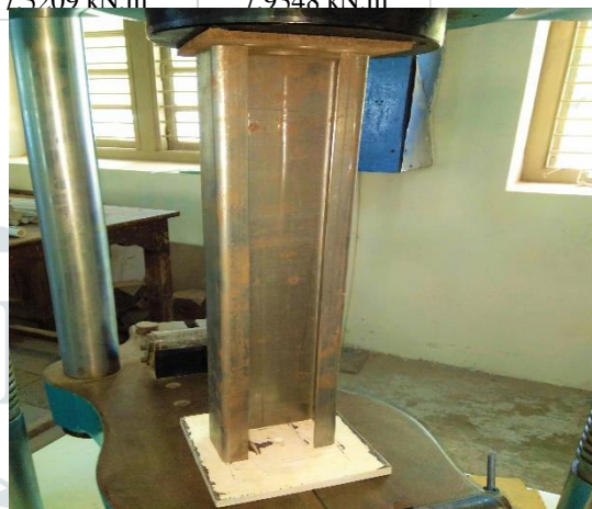
Fig 5. Channel Fix in UTM
