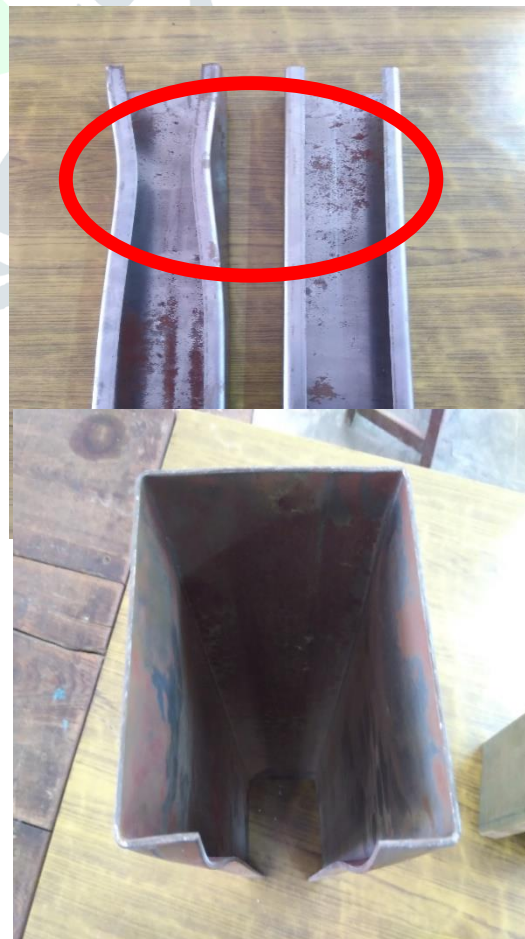
Fig 6. Digital UTM 7. Failure Shape Channel section size 100x50x3x15
