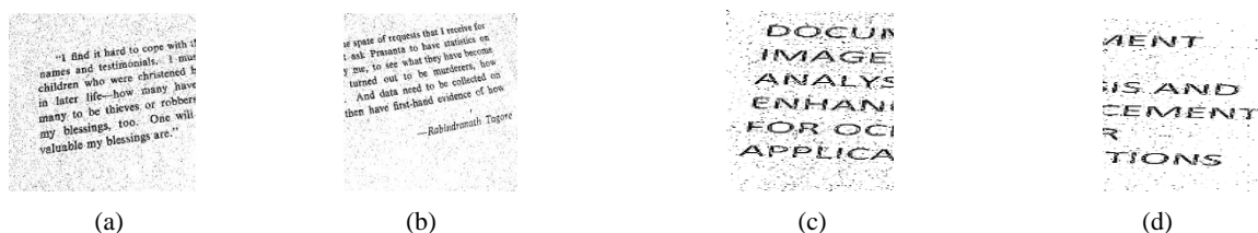
Figure 3. Binarized image using adaptive thresholding with improper window size: (a), (b) Binarized left half and right half of Fig. 1(a) with a neighborhood 7 \times 7 & constant 0.1. (c), (d) Binarized left half and right half of Fig. 1(b) with a neighborhood 7 \times 7 & constant 0.1
