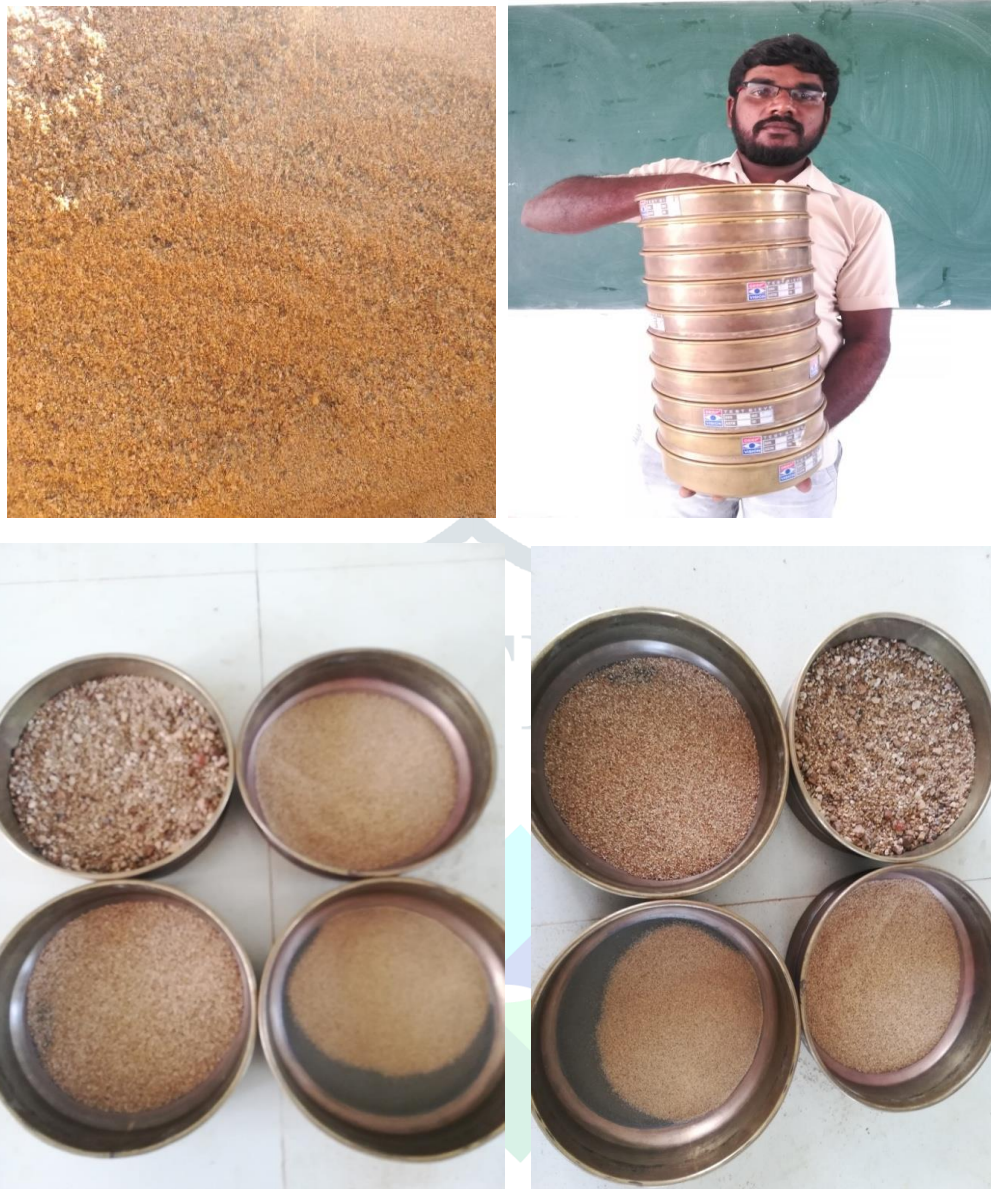
Plate 2: - Sand grain Analysis of Grading in sedimentology laboratory A) Sand collected from Papagni River; B) sand grading by sieve analysis using various sieve sizes. C&D) coarse medium fine and very fine grade sand from two sites.
