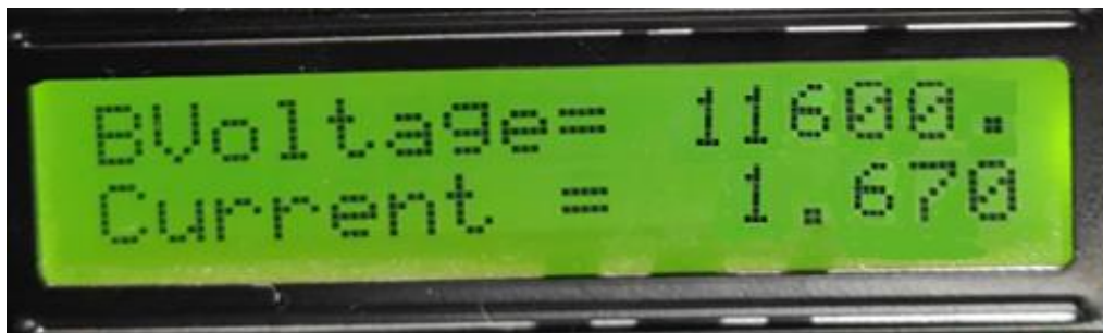
Fig. Voltage (mV) and Current (A) reading of Battery
