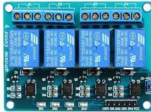
Fig 3.2.2: A Relay Module with four 5V Relays
