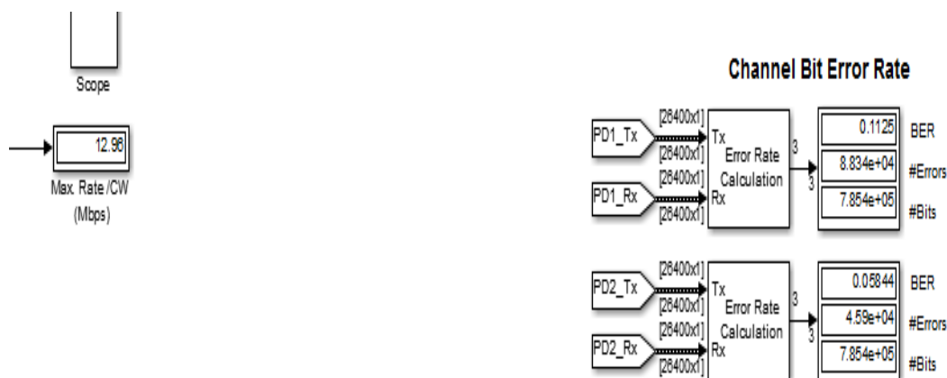
Fig.5: Result (Speed and BER) as obtained for Rayleigh Fading Channel
