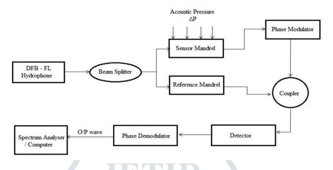
Figure: A basic block diagram of DFB - FL hydrophone.
