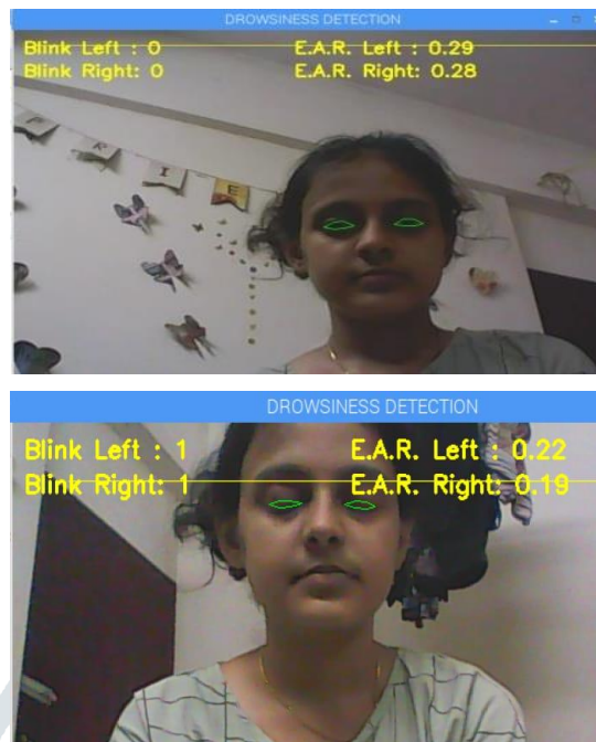
Figure 4 : Detection of eye blinking and Calculating EAR for blinked eyes
