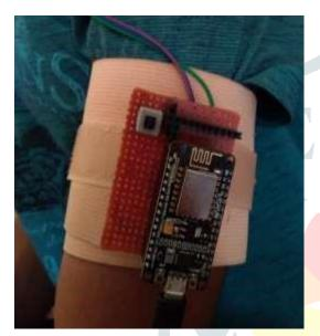
Fig 5 : Sensor Node to Sense Temperature
