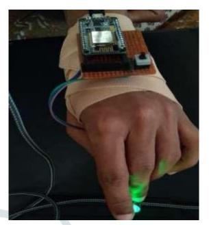
Fig 6 : Sensor Node to Sense Pulse rate
