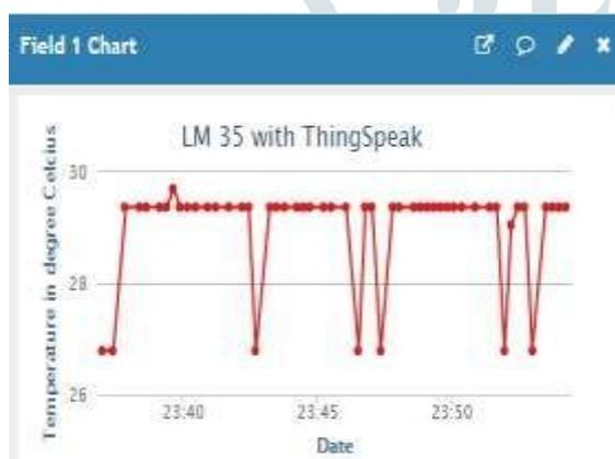
Fig 8 : LM35 Output on Thingspeak
