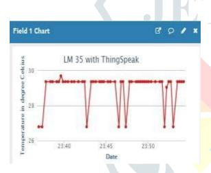
Fig 8 : LM35 Output on Thingspeak
